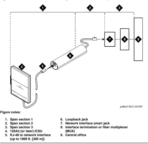
10 9 6 120A prdfcs4 KLC 012797 Figure notes: 1. Span section 1 6. Loopback jack
